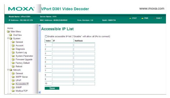
Accessible IP Settings allows you to add or remove "Legal" remote host IP addresses to prevent unauthorized access. Access to the VPort is controlled by IP address. That is, if a host's IP address is in the accessible IP table, then the host will be allowed access to the VPort. The Administrator can allow one of the following cases by setting this parameter:
