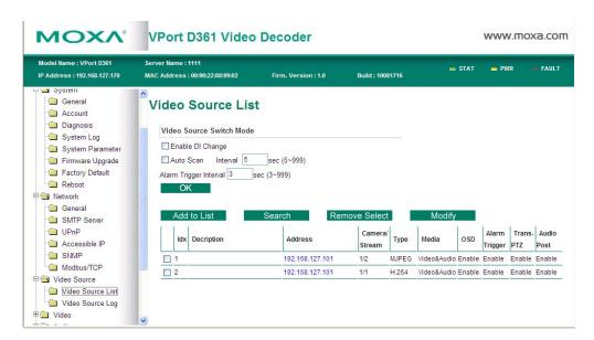
A maximum of 64 video sources can be added to the VPort D361's video source list. The Administrator can configure the video source operation settings on this page.
