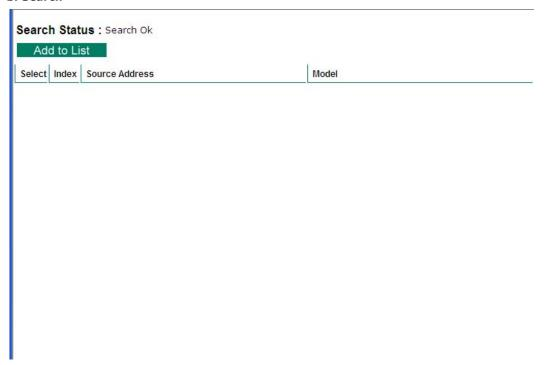
The **Search** function is used to search for video source devices on the network that are on the same domain network as the computer that you are searching from. After the search, the Administrator can select the video source device and then click **Add to List** to add this video source to the video source list. After that, the Administrator can use the **Modify** function to edit the video source configurations.
