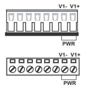
**STEP 1:** Insert the negative/positive DC or AC wires into the V-/V+ terminals.
