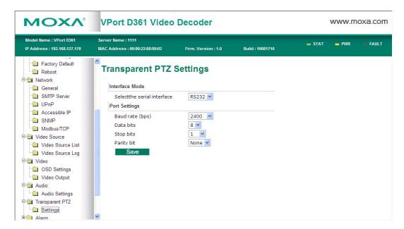
The VPort D361 supports the transparent PTZ control function, which means the user can connect a legacy PTZ control panel to the VPort D361's PTZ port to control the PTZ camera connected to the VPort video encoder. It is not necessary to install PTZs.
