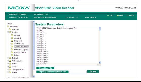
NOTE The system parameter import/export functions allow the Administrator to back up and restore system configurations. The Administrator can export this sys\_config.ini file (in a special binary format) for backup, and import the sys\_config.ini file to restore the system configurations of the VPort. System configurations will be changed immediately after the VPort is rebooted.
