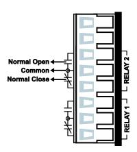
The Relay Output can be set up for: System alarm: In this case, network disconnected. Event alarm: Digital inputs.
