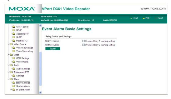
**NOTE** The relays will not be triggered when the Override Relay 1 warning setting and Override Relay 2 warning setting boxes are checked. Un-check these 2 boxes to allow the relays to be triggered.
