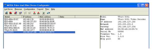
**NOTE** Broadcast Search can only search for devices connected to the same LAN domain as the VPort. If your devices are located on a different LAN domain, use the Specify IP Address function to search for the device by keying in the IP address.
