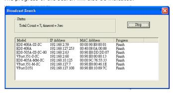
3. When the search has ended, the Model Name, MAC address, and IP address of the EDS switches and the VPorts will be listed in the **Utility** window.
